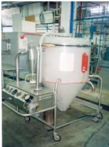
**Fig. 10.4 A laboratory spray dryer**
