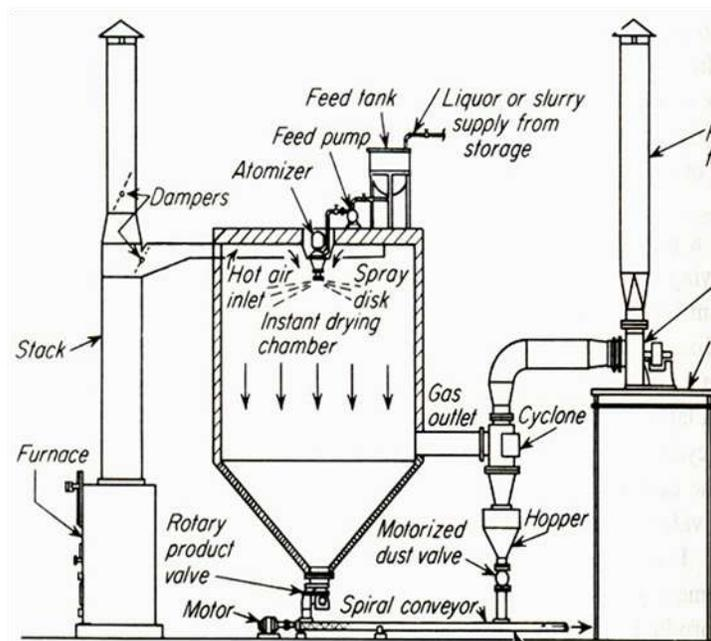
**Fig. 10.2 Components of a spray drying system**
