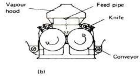
Fig. 10.9 Two common configurations of drum dryers
