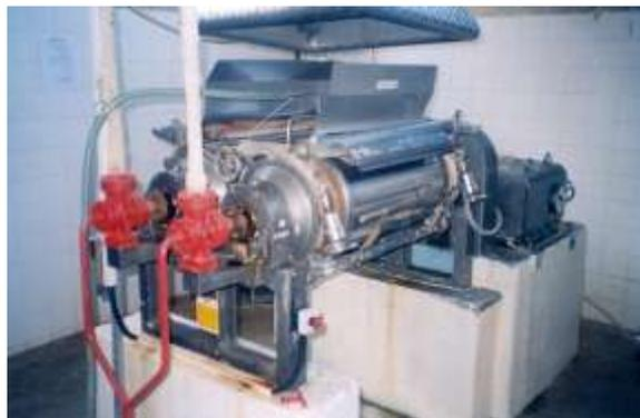
Fig. 10.6 A laboratory scale double drum dryer
