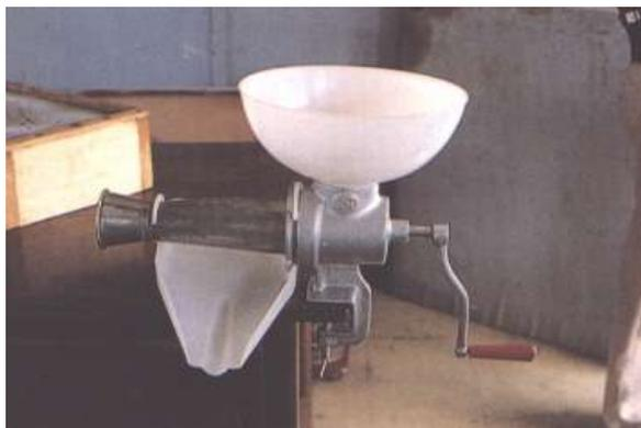
**Fig. 11.1 Hand operated pulp extractor**
