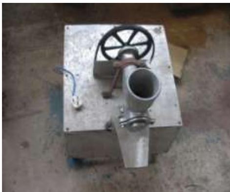
**Fig. 11.2 Motor operated pulper**
