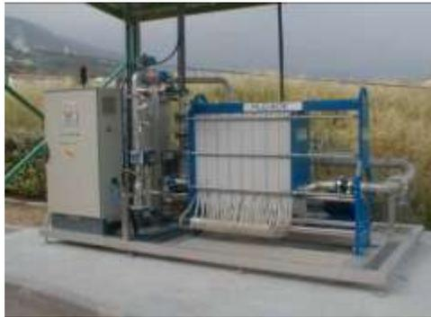
**Fig. 12.10 Plate and frame module in waste water system**
