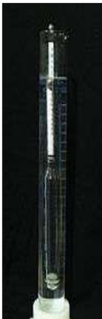
**Fig. 2.2 A lactometer immersed in a cylinder**
