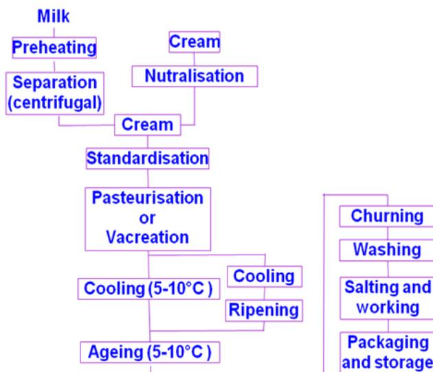
Fig. 3.6 Flow chart for preparation of butter
