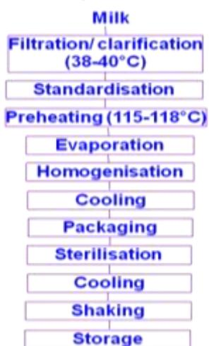
**Fig. 3.11** Flow chart for preparation of evaporated milk
