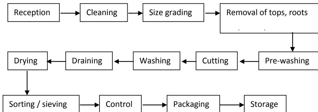
**Fig. 3.12: Preparation of dehydrated onion**
