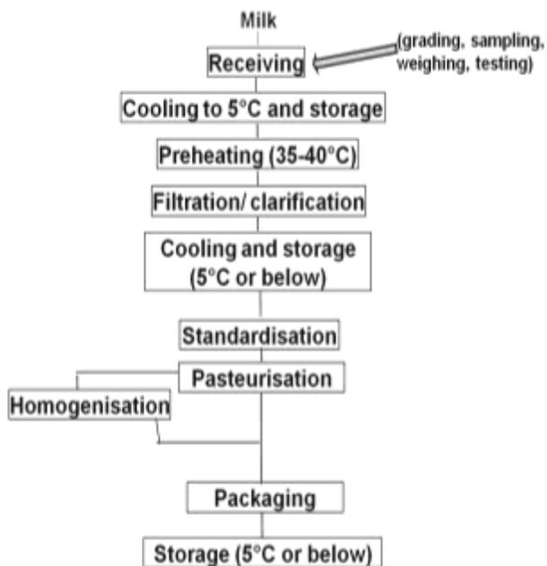
**Fig. 3.2 Flow chart for preparation of pasteurized milk**
