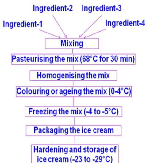
Fig. 3.7 Flow chart for preparation of ice cream
