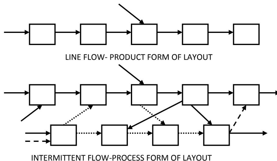
**Fig. 3.14 Product form and process form of layout**
