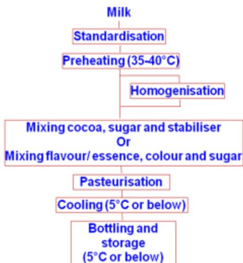
**Fig. 3.4 Flow chart for preparation of flavoured milk**
