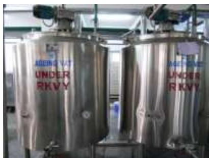
**Fig.4.9 Processing tanks for milk**
