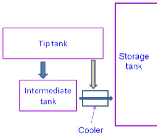
**Fig. 4.3 Arrangement of tanks in milk reception section**
