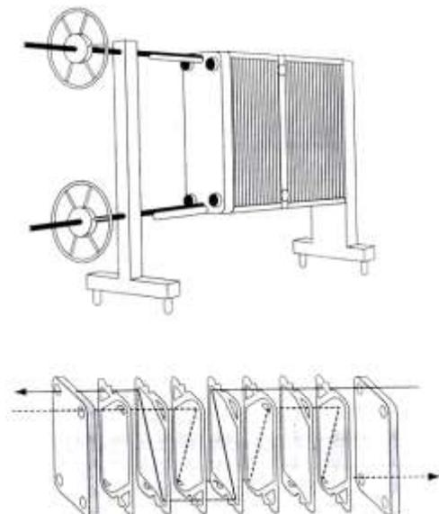
**Fig. 5.4 Plate heat exchanger**
