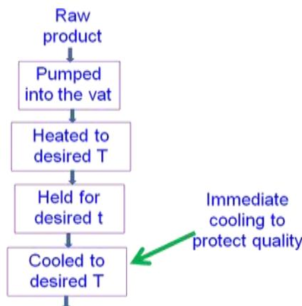
**Fig. 5.1 Basic operations in a vat pasteuriser**
