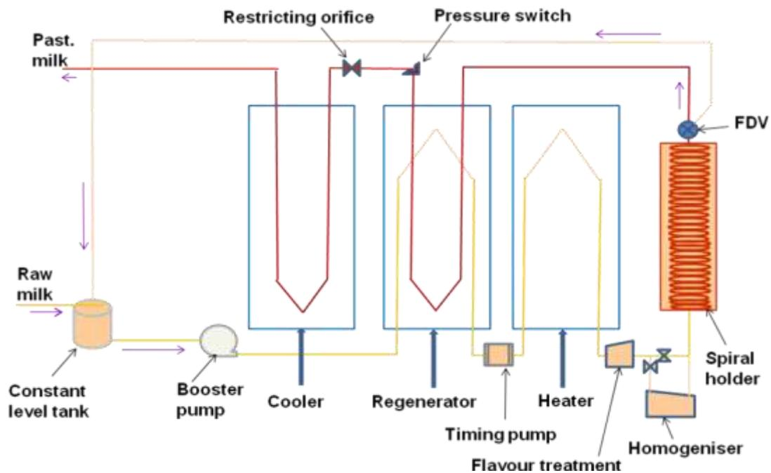
**Fig. 5.10 Homogenizer incorporated in HTST pasteurization system**
