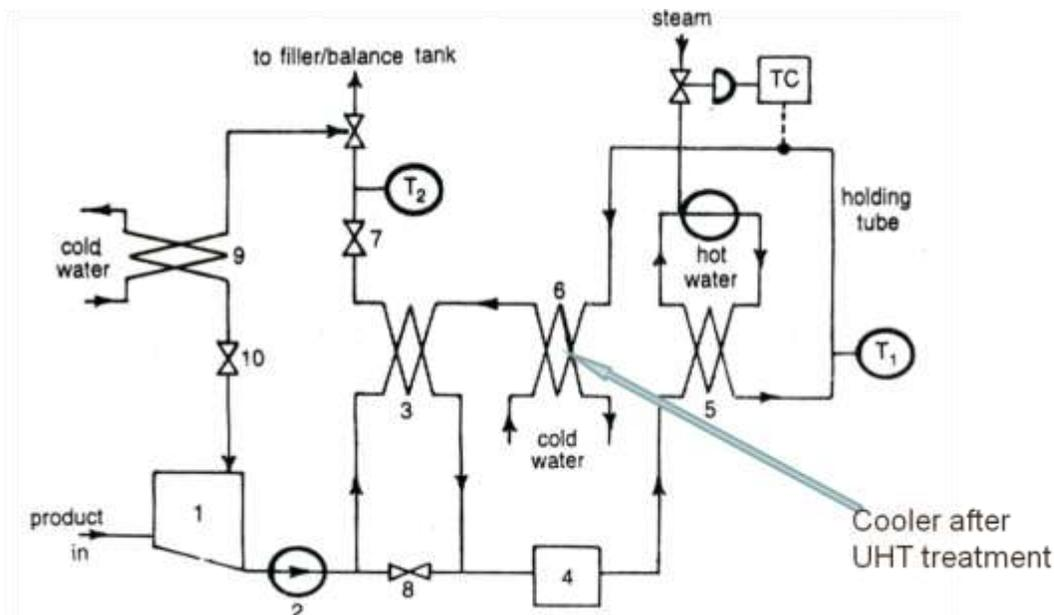
**Fig. 6.10 UHT sterilization process (indirect heating type)**
