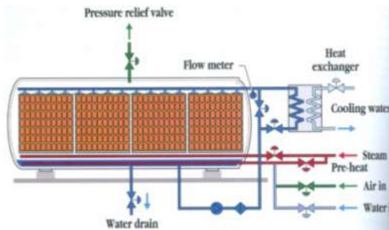
**Fig. 6.5 Water spray or cascading water retort**
