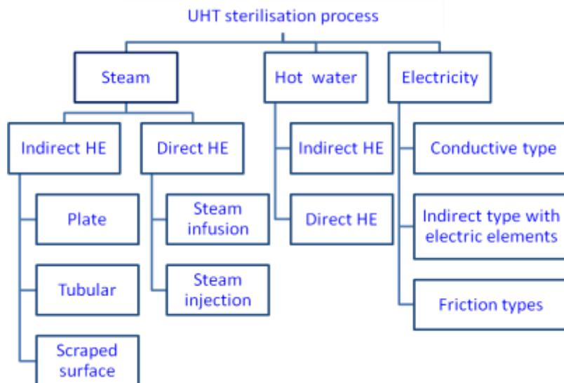
**Fig. 6.9 Classification of UHT sterilization process**
