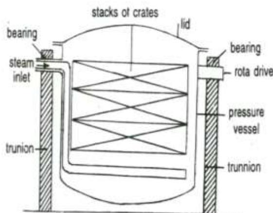
**Fig. 6.6 Rotary batch sterilizer**
