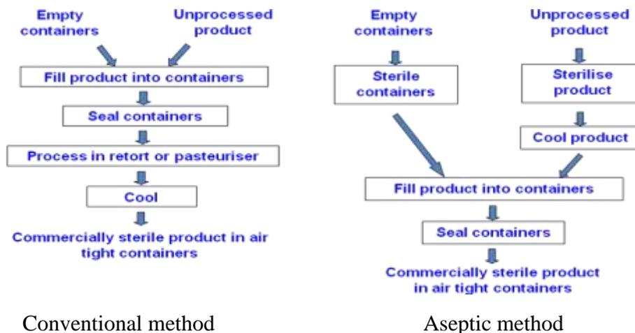
Fig. 6.1 Difference between conventional and aseptic processing methods
