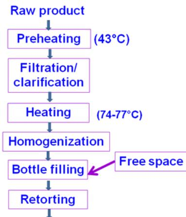
**Fig. 6.2 In-bottle sterilization process**
