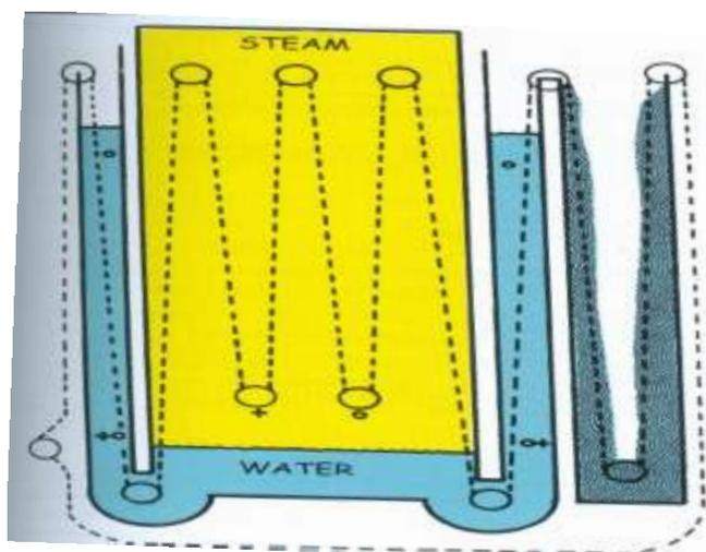
**Fig. 6.7 Hydrostatic retort**
