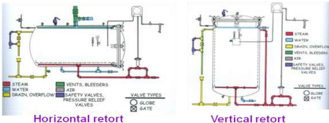
**Fig. 6.4 Basic parts of retort**
