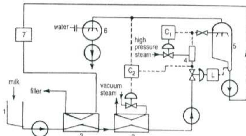
**Fig. 6.13 UHT sterilization process (direct heating type)**
