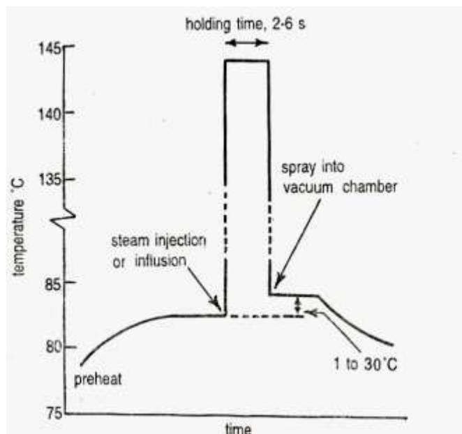
**Direct heating injection type system**
