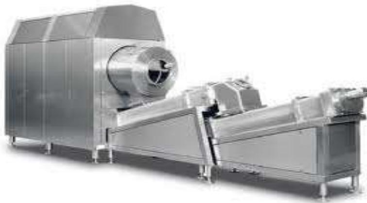
**Fig. 9.10 Continuous Butter Churn (Exterior view)**
