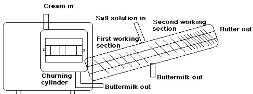
**Fig. 9.9 Schematic diagram of a continuous Butter Churn**
