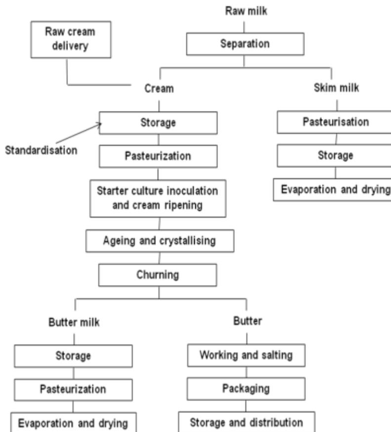
**Fig. 9.5 Butter making process**
